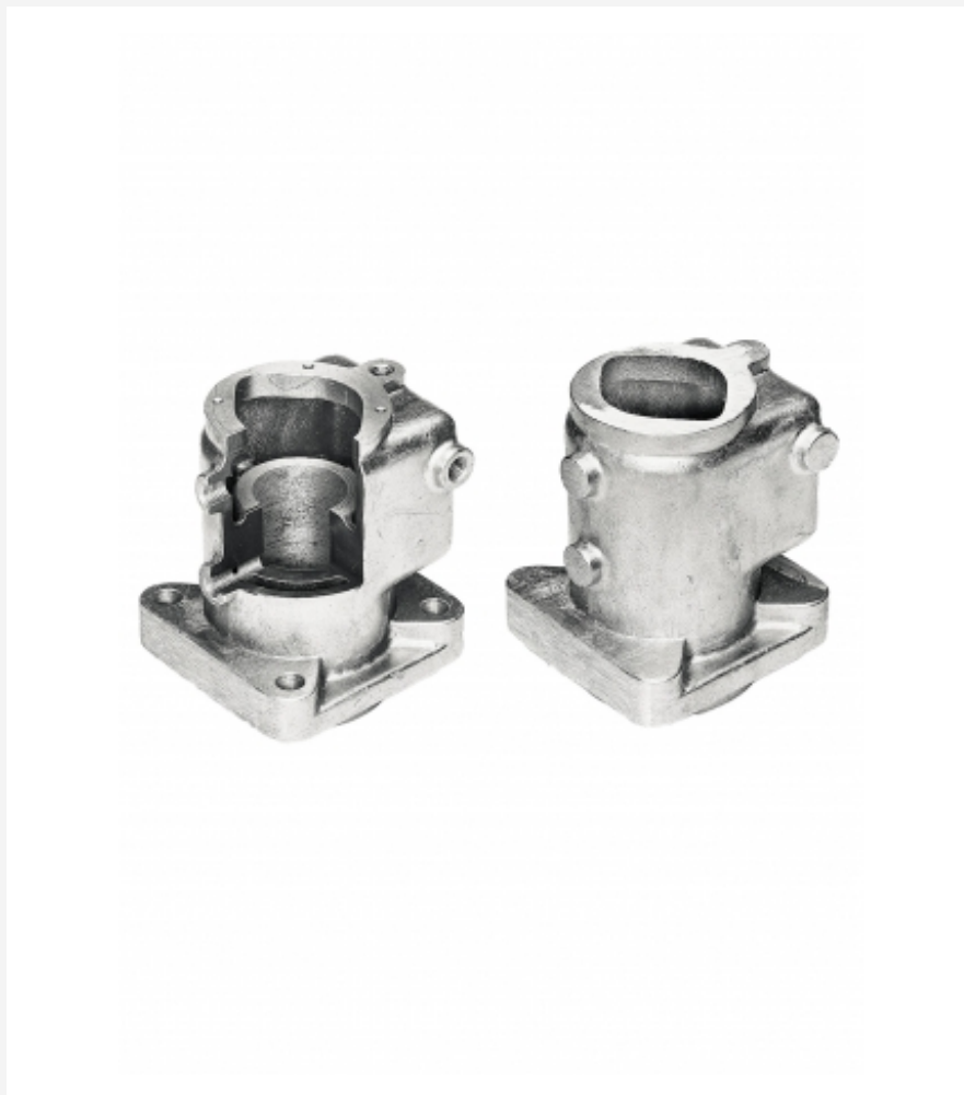
Machined (left) and raw casting (right)
